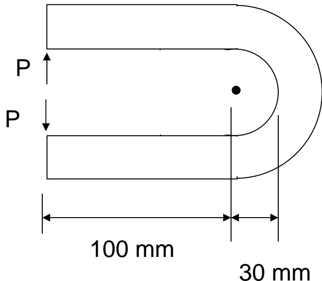
For a square 50x50 mm cross-section, find the maximum tensile and compressive stress if  $P = 9.5 \text{ kN}$  and plot the total stress across the cross-section
