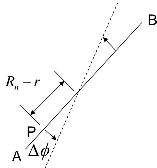
$$e_{\theta\theta} = \frac{\Delta l}{l} = \frac{(R_n - r)\Delta\phi}{r\Delta\theta} = \omega \left( \frac{R_n}{r} - 1 \right)$$
